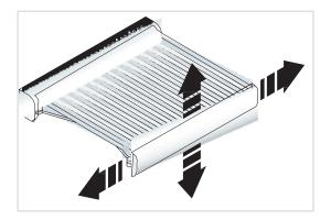
The motion sensor detects horizontal, vertical and lateral movement of the awning.
