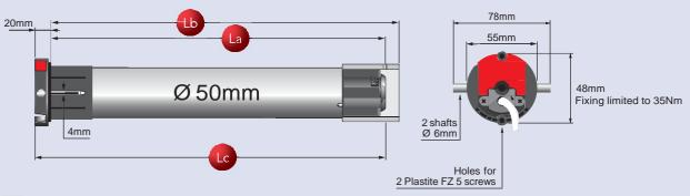
(a): Length between the end and the drilling point of the tube
