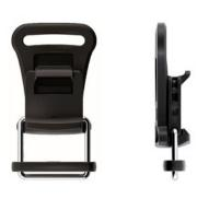
Opening mechanism Webbing width  $25\,mm$ Weight ca. 14 g Dimensions (L×W×H) 44,5 × 33,9 × 12,4 mm Material PA66GF15 Static breaking load 40 kg Colour black
