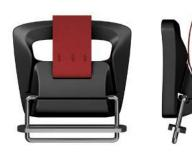
Opening mechanism lift Webbing width 40 mm Weight ca. 40 g Dimensions (L×W×H) 48,0 × 58,2 × 17,3 mm Material PA66GF15, stainless steel, aluminium Static breaking load 100 kg (with glide bar); 200 kg (withou
