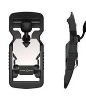
Opening mechanism lift Webbing width 25 mm Weight ca. 25 g Dimensions (L×W×H) 72,0 × 34,0 × 14,0 mm Material PA66GF30, stainless steel Static breaking load 70 kg Colour black/stainless steel Assembly strap, single bar, ladderlock
