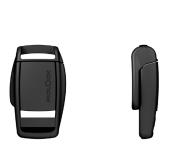
Opening mechanism slide laterally Webbing width 15 mm Webbing thickness 1,6 mm Weiaht ca. 11 g Dimensions (L×W×H) 46,3 × 28,0 × 13,2 mm Material PA6GFCF30, PP Static breaking load 65 kg Colour black Assembly
