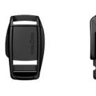
Opening mechanism slide laterally Webbing width 15 mm Webbing thickness (single layered; double layered) 2,5 mm; 1,3 mm Weight ca. 12 g Dimensions (L×W×H) 46,8 × 28,0 × 13,4 mm Material PAGF40, PP Static breaking load 75 kg Colour black Assembly
