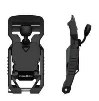
Opening mechanism lift Webbing width 25 mm Weight ca. 27 g Dimensions (L×W×H) 72,8 × 34,2 × 16,0 mm Material PA66GF30, stainless steel Static breaking load 70 kg
