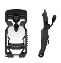
Opening mechanism lift Webbing width 25 mm Weight ca. 27 g Dimensions (L×W×H) 72,8 × 34,2 × 16,0 mm Material PA66GF30, stainless steel Static breaking load 70 kg Colour black/stainless steel Assembly strap, screwing, ladderlock
