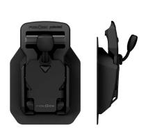
Opening mechanism lift Webbing width 25 mm Weight ca. 26 g Dimensions (L×W×H) 69,5 × 47,2 × 16,0 mm Material PA6, PA66GF15, stainless steel Static breaking load up to 60 kg Colour black Assembly sewing, strap, ladderlock
