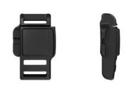
Opening mechanism slide laterally Webbing width 15 mm Weight ca. 11 g Dimensions (L×W×H) 46,4×29,8×13,9 mm Material PA66GF30 Static breaking load 55 kg
