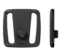
Opening mechanism defined by female part Webbing width 50 mm Weight ca. 21 g Dimensions (L×W×H) 62,8 × 61,6 × 13,0 mm Material PA66GF15 Static breaking load 37 kg Colour black
