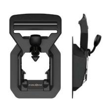
Opening mechanism lift Webbing width 40 mm Weight ca. 29 g Dimensions (L×W×H) 80,0 × 47,2 × 16,0 mm Material PA6, PA66GF30, stainless steel Static breaking load up to 60 kg Colour black/stainless steel Assembly
