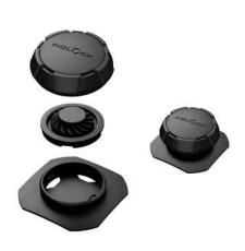
Opening mechanism lift Weight ca. 11 g Dimensions 37 x 37 mm (L x W of total base) Dimensions (Ø; height) 32,8 mm; 10,5 mm (handle) Rope diameter 1,2 - 2,75 mm Material PA66GF15, ABS, PA6 Static breaking load 20 kg (handle) Colour black Assembly clip together, sewing, rope For material thinkness up to 3,0 mm Tools for assembly TOOL 30
