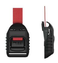
Opening mechanism lift Webbing width 25 mm Weight ca. 23 g Dimensions (L×W×H) 106,6 × 37,4 × 14,6 mm Material PA6, POM, stainless steel Static breaking load 45 kg Colour black Assembly
