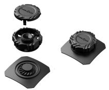
Opening mechanism lift Weight ca. 7 g Dimensions 35 x 35 mm (L x W of total base) Dimensions (Ø; height) 26,4 mm: 6,2 mm (handle) Rope diameter 1 - 1,6 mm Material PA6, PP Static breaking load 16 kg Colour black Assembly sewing, rope For material thinkness up to 1,3 mm
