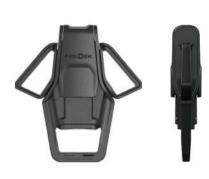
Opening mechanism single press Webbing width 30 mm Weight ca. 57 g Dimensions (L×W×H) 97,3 × 83,1 × 22,2 mm Material PA66GF30, PA66GF15, POM Static breaking load 40 kg Colour black | grey
