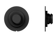
Opening mechanism defined by female part Weight ca. 6 g Dimensions (Ø; height) 40,8 mm; 12,6 mm Punch hole for assembly 26 mm Material PA6 Static breaking load 30 kg
