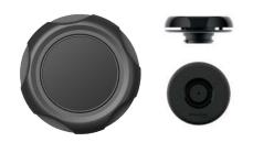
Opening mechanism turn Weight ca. 37 g Dimensions 50 mm (Ø female); 51,0 mm (Ø handle) Height (female: male) 9,8 mm; 23,9 mm Punch hole for assembly female: 36,0 mm; male: 27,0 mm Material PA66GF15 Static breaking load 44 kg Colour black Assembly threaded ring (included) For material thinkness female and male: 1,0 - 2,6 mm Tools for assembly
