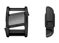
Opening mechanism slide laterally Webbing width 25 mm Weight ca. 25 g Dimensions (L×W×H) 50,2 × 40,3 × 15,4 mm Material PA66GF15, stainless steel Static breaking load 25 kn
