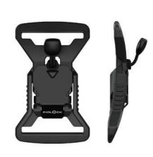
Opening mechanism lift Webbing width 40 mm Weight ca. 26 g Dimensions (L×W×H) 80,0 × 49,0 × 13,5 mm Material PA66GF30, stainless steel Static breaking load 70 kg Colour black Assembly
