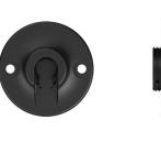
Opening mechanism slide Weight ca. 5 g Dimensions (Ø; height) 42,5 mm; min. 5,5 mm Punch hole for assembly 20,0 mm Material PA66GF15 Static breaking load 2 kg Colour black Assembly rivets (not included)
