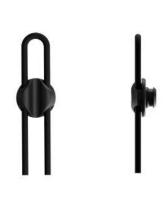
Opening mechanism defined by female part Weight ca. 2 g Dimensions 18,5 mm (Ø) Material PA66GF15 Static breaking load 2 kg Colour black Assembly clip together, screw thread, rope For material thinkness rope: 3,0 mm Tools for assembly front: TOOL 4; back: TOOL 18
