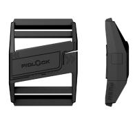
Opening mechanism slide laterally Webbing width 40 mm Weight ca. 29 g Dimensions (L×W×H) 66,8 × 49,0 × 16,2 mm Material PA66GF15 Static breaking load
