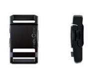
Opening mechanism slide laterally Webbing width 20 mm Weight ca. 15 g Dimensions (L×W×H) 46,8 × 27,5 × 13,1 mm Material PAGF40, ABS Static breaking load 75 kg Colour black Assembly
