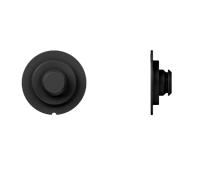
Opening mechanism defined by female part Weight ca. 4 g Dimensions (Ø; height) 31,8 mm; 10,2 mm Punch hole for assembly 22 mm Material PA6 Static breaking load 15 kg Colour black Assembly sewing For material thinkness up to 2,5 mm
