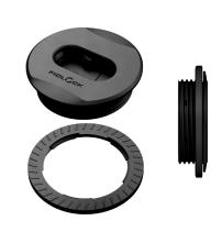
Opening mechanism slide laterally Weight ca. 15 g Dimensions 50 mm (Ø threaded ring) Dimensions (Ø; height) 45 mm; 13 mm Punch hole for assembly 38,0 mm Material PA66GF15, stainless steel (magnetized) Static breaking load 30 kg Colour black Assembly threaded ring (included) Tools for assembly front: TOOL 31; back TOOL 3
