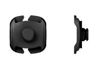
Opening mechanism defined by female part Webbing width 25 mm Weight ca. 6 g Dimensions (L×W×H) 37,7 × 36,0 × 13,7 mm Material PA66GF Static breaking load 20 kg Colour black
