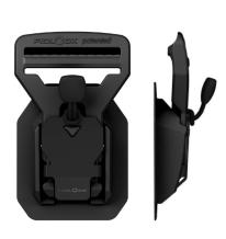
Opening mechanism lift Webbing width 40 mm Weight ca. 29 g Dimensions (L×W×H) 80,0 × 47,2 × 16,0 mm Material PA6, PA66GF30, stainless steel Static breaking load up to 60 kg Colour black
