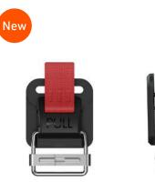
Opening mechanism lift Webbing width 25 mm Weight 16,00 g Dimensions (L×W×H) 49 × 34 × 12 mm (incl. D-ring) Material PA6, PA6GF, epoxy, NdFeB, stainless steel, fabric Colour black
