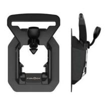
Opening mechanism lift Webbing width 40 mm Weight ca. 26 g Dimensions (L×W×H) 72,3 × 47,2 × 16,0 mm Material PA6, PA66GF30, stainless steel Static breaking load up to 60 kg Colour
