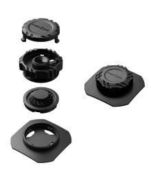
Opening mechanism lift Weight ca. 9 g Dimensions 37 x 37 mm (L x W of total base) Dimensions (Ø; height) 26,4 mm; 5,1 mm (handle) Rope diameter 1 - 1,6 mm Material PA6, PP Static breaking load 16 kg (handle) Colour black Assembly clip together, sewing, rope For material thinkness up to 3,0 mm Tools for assembly TOOL 30
