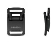
Opening mechanism lift Webbing width 20 mm Weight ca. 8 g Dimensions (L×W×H) 43,5 × 26,8 × 10,4 mm Material PA66GF15 Static breaking load 15 kg Colour black Assembly
