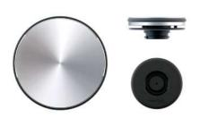
Opening mechanism turn Weight ca. 46 g Dimensions 50 mm (Ø female); 52,0 mm (Ø handle) Height (female: male) 9,8 mm; 21,2 mm Punch hole for assembly female: 36,0 mm; male: 27,0 mm Material PA66GF15, aluminium Static breaking load 44 kg Colour aluminium anodized Assembly threaded ring (included) For material thinkness female and male: 1,0 - 2,6 mm Tools for assembly female: TOOL 2/TOOL 3/TOOL 22; male: TOOL 1/ T00L3/T00L22
