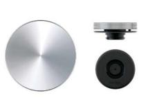
Opening mechanism turn Weight ca. 45 g Dimensions 50 mm (Ø female); 50,0 mm (Ø handle) Height (female; male) 9,8 mm; 20,8 mm Punch hole for assembly female: 36,0 mm; male: 27,0 mm Material PA66GF15, aluminium Static breaking load 44 kg Colour aluminium anodized Assembly threaded ring (included) For material thinkness female and male: 1,0 - 2,6 mm Tools for assembly female: TOOL 2/TOOL 3/TOOL 22; male: TOOL 1/ T00L3/T00L22
