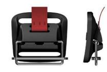
Opening mechanism lift Webbing width 40 mm Weight ca. 35 g Dimensions (L×W×H) 49,1×53,9×18,0 mm Material PA66GF15, stainless steel Static breaking load 40 kg Assembly
