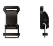
Opening mechanism lift Webbing width 15 mm Weight ca. 10 g Dimensions (L×W×H) 32,2 × 23,0 × 11,9 mm (incl. D-ring) Material PA6, PAGF40, stainless steel Static breaking load 50 kg Colour black Assembly strap, glide bar, single bar
