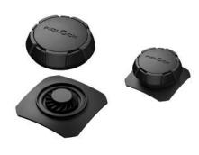
Opening mechanism lift Weight ca. 13 g Dimensions 35 x 35 mm (L x W of total base) Dimensions (Ø; height) 32,8 mm; 10,5 mm (handle) Rope diameter 1,2 - 2,75 mm Material PA6, PA6GF15, ABS Static breaking load 20 kg Colour black Assembly sewing, welding
