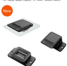
Opening mechanism flip lever Weight ca. 27 g Dimensions (L×W×H) female: 29,2 × 59,4 × 12,3 mm; male: 43,6 × 35,8 × 14,0 mm Material PA66GF30, PA66GF15, stainless steel, PA6, stainless steel (Zn coated) Static breaking load 100 kg Colour black Assembly rivets or screws (not included), clip in (see
