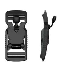
Opening mechanism lift Webbing width 25 mm Weight ca. 26 g Dimensions (L×W×H) 79,6 × 34,2 × 11,6 mm Material PA66GF, stainless steel Static breaking load 70 kg Colour black Assembly ladderlock, strap
