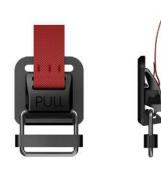
Opening mechanism pull Webbing width 25 mm Weight ca. 13 g Dimensions (L×W×H) 49,2 × 34 × 11,8 mm (incl. D-ring) Material PA6, PA66GF15, stainless steel Static breaking load 30 kg Colour black Assembly
