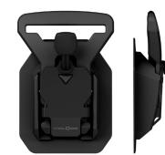
Opening mechanism lift Webbing width 40 mm Weight ca. 26 g Dimensions (L×W×H) 72,3 × 47,2 × 16,0 mm Material PA6, PA66GF30, stainless steel Static breaking load up to 60 kg Colour black Assembly sewing, strap, single bar
