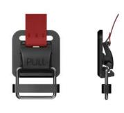
Opening mechanism lift Webbing width 25 mm Weight ca. 21 g Dimensions (L×W×H) 33,9 × 34,0 × 11,8 mm Material PA6, aluminium Static breaking load 200 kg Colour black Assembly strap, single bar, glide bar
