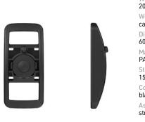
Opening mechanism slide Webbing width 20 mm Weight ca. 9 g Dimensions (L×W×H) 60,0 × 28,0 × 12,0 mm Material PA66GF15 Static breaking load 15 kg Colour black Assembly strap
