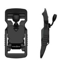
Opening mechanism lift Webbing width 25 mm Weight ca. 25 g Dimensions (L×W×H) 72,0 × 34,0 × 14,0 mm Material PA66GF30, stainless steel Static breaking load 70 kg
