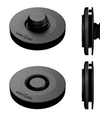
Opening mechanism defined by female part Weight ca. 16 g Dimensions (Ø; height) 50 mm; 12,5 mm (retracted) Punch hole for assembly 35,6 mm Material PA66GF Static breaking load 30 kg Colour black Assembly screw thread Tools for assembly front: no tool; back: TOOL 2/TOOL 3/TOOL 22
