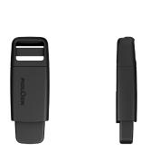
Opening mechanism push Webbing width 15 mm Weight ca. 8 g Dimensions (L×W×H) 58,0 × 21,2 × 11,1 mm Material PA66GF15 Static breaking load 2 kg Colour black Assembly strap, ladderlock
