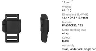
Opening mechanism slide laterally Webbing width 15 mm Weight ca. 12 g Dimensions (L×W×H) 46,4 × 29,8 × 13,9 mm Material PA6GFCF30, ABS Static breaking load 65 kg Colour black
