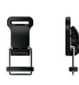
Opening mechanism lift Webbing width 15 mm Weight ca. 10 g Dimensions (L×W×H) 51,7 × 21,6 × 11,9 mm (incl. D-ring) Material PA6, PAGF40, stainless steel Static breaking load 50 kg Colour black Assembly strap, glide bar, single bar
