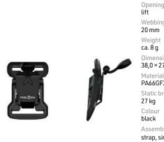
Opening mechanism Lift Webbing width 20 mm Weight ca. 8 g Dimensions (L×W×H) 38,0 × 27,4 × 9,3 mm Material PA66GF30, stainless steel Static breaking load 27 kg Colour black Assembly strap, single bar
