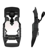
Opening mechanism lift Webbing width 20 mm Weight ca. 23 g Dimensions (L×W×H) 74,0 × 34,2 × 13,5 mm Material PA66GF30, stainless steel Static breaking load 70 kg Colour black/stainless steel Assembly strap, single bar, ladderlock
