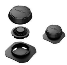
lift Weight ca. 11 g Dimensions 37 x 37 mm (L x W of total base) Dimensions (Ø; height) 32,8 mm; 10,5 mm (handle) Rope diameter 1,2 - 2,75 mm Material PA66GF15, ABS, PA6 Static breaking load 20 kg (handle) Colour black Assembly clip together, sewing, rope For material thinkness up to 3,0 mm Tools for assembly TOOL 30
