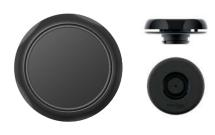
Opening mechanism turn Weight ca. 43 g Dimensions 50 mm (Ø female); 49,6 mm (Ø handle) Height (female: male) 9,8 mm; 28,0 mm Punch hole for assembly female: 36,0 mm; male: 27,0 mm Material PA66GF15 Static breaking load 44 kg Colour black Assembly threaded ring (included) For material thinkness female and male: 1,0 - 2,6 mm Tools for assembly
