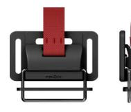
Opening mechanism lift Webbing width 40 mm Weight ca. 28 g Dimensions (L×W×H) 35,5 × 63,3 × 12,1 mm Material PA6, PA66GF15, stainless steel Static breaking load 50 kg Colour black Assembly strap, glide bar, tri-glide, single bar
