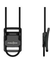
Opening mechanism lift Webbing width 20 mm Weight ca. 7 g Dimensions (L×W×H) 37,3×26,8×8,5 mm Rope diameter 3,0 mm Material PA66GF15 Static breaking load 3 kg Colour black
