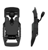
Opening mechanism lift Webbing width 20 mm Weight ca. 23 g Dimensions (L×W×H) 74,0 × 34,2 × 13,5 mm Material PA66GF30, stainless steel Static breaking load 70 kg
