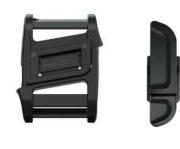
Opening mechanism slide laterally Webbing width 25 mm Weight ca. 21 g Dimensions (L×W×H) 50,0 × 40,1 × 15,4 mm Material PA66GF15 Static breaking load 25 kg Colour black Assembly strap, single bar, ladderlock
