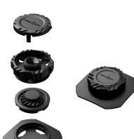
Weight ca.9g Dimensions 37 x 37 mm (L x W of total base) Dimensions (Ø; height) 26,4 mm; 5,1 mm (handle) Rope diameter 1 - 1,6 mm Material PA6, PP Static breaking load 16 kg (handle) Colour black Assembly clip together, sewing, rope For material thinkness up to 3,0 mm Tools for assembly TOOL 30
