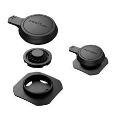
Opening mechanism lift Weight ca. 12 g Dimensions 37 x 37 mm (L x W of total base) Dimensions (Ø; height) 34,0 mm; 10,49 mm (handle) Rope diameter 1,2 - 2,75 mm Material PA6, PA6GF15, ABS, TPU Static breaking load 20 kg (handle) Colour black Assembly sewing, clip together, rope For material thinkness up to 3,0 mm Tools for assembly TOOL 30
