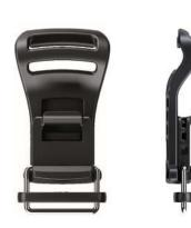
Opening mechanism lift Webbing width 25 mm Weight ca. 15 g Material PA666F15 Static breaking load 40 kg Colour black Assembly strap, glide bar, ladderlock
