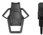
Opening mechanism double press Webbing width 25 mm Weight ca. 57 g Dimensions (L×W×H) 97,7 × 83,1 × 22,2 mm Material PA66GF30, PA66GF15, POM Static breaking load 40 kg Colour black | grey Assembly
