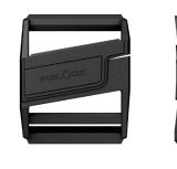
Opening mechanism slide laterally Webbing width 40 mm Weight ca. 28 g Dimensions (L×W×H) 57,6 × 49,0 × 16,5 mm Material PA66GF15 Static breaking load 30 kg Colour black Assembly strap, ladderlock, single bar
