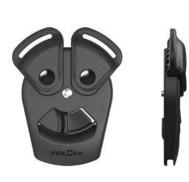
Opening mechanism push & slide Webbing width 25/40 mm Weight ca. 50 g Dimensions (L×W×H) 96,6 × 77,0 × 13,5 mm Material PA66GF15, ABS, steel (zinc coated), stainless steel Static breaking load 40 kg Colour black Sector children, transportation
