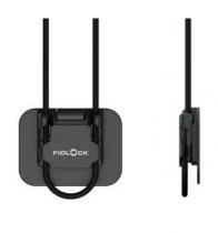
Opening mechanism lift Weight ca. 7 g Dimensions (L×W×H) 32,4×42,8×8,6 mm Rope diameter 3.0 mm Material PA66GF15 Static breaking load 3 kg Colour black Assembly
