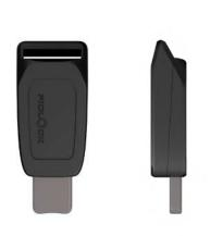
Opening mechanism push Webbing width 25 mm Weight ca. 18 g Dimensions (L×W×H) 78,0 × 32,0 × 16,0 mm Material PA66GF15 Static breaking load 30 kg Assembly strap, ladderlock
