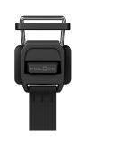
Opening mechanism lift Weight ca.9g Dimensions (L×W×H) 41,7 (incl. D-ring) × 31,0 × 10,3 mm Material PA6, stainless steel Colour black Assembly strap, sewing, glide bar
